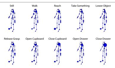
Figure 6: Joints selected by binary tests assigned to nodes of the Hough forest, where size of the plotted joint on the stick figure corresponds to frequency of selection. Note that each test uses two joints as the relational pose feature.
